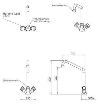
Supplied with two inlet stainless steel hoses 300mm long 3/8"BSP female connections
